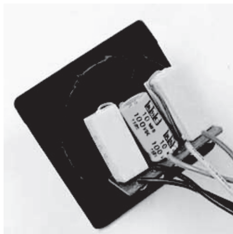
A typical crossover unit from a loudspeaker. The frequency is divided up by inductors and capacitors and then sent on to the woofer, tweeter and mid-range driver.
